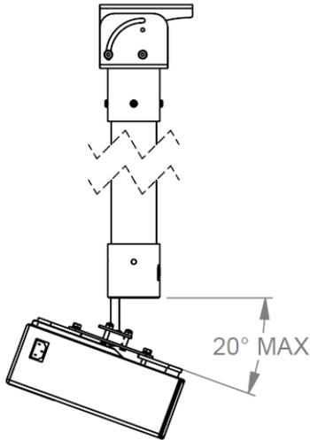
DETACHABLE & ROTATABLE TOP MOUNT PROVIDES FLEXIBILITY FOR A VARIETY OF MOUNTING CONFIGURATIONS
